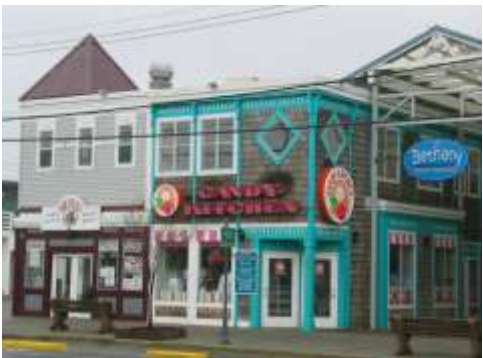
Window variation: Large storefront windows below with smaller decorative windows above Entry doors: recessed corner doors provide relief
