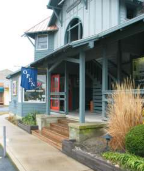
Example of porch as entry element to multiple stores, detail with exposed structure, unique bracketing and open CIRCULAR "WINDOW".
